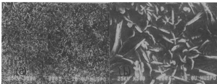
FIGURE 4 (a) A uniform, densely packed growth of fine-grained secondary crystals after 3 min of nickel-activated phosphating of CRS etched with dilute HCl. (b) A mixed secondary growth of platelet and dendritic crystals after 15 min of nickel-activated phosphating of CRS etched with dilute HCl.
